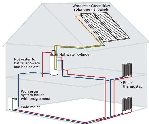
**System boiler layout and solar water heating system**
