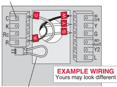
Remove jumper loop **ONLY** if you have both **R** and **Rc** wires.
